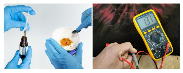
Figure 3: The chemical products used to functionalize our textile, Pyrrole and Iron Chloride (left). After functionalization, the textile is conductive, except where it was tied (right).
