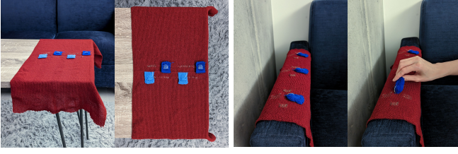
Figure 17: Furniture covering. Leveraging digital design and fabrication pipeline, MagKnitic can be integrated into furniture coverings, including table cloth, and sofa coverings, for diverse user interactions with passive haptic feedback. Using scenarios include tangible and interactive task checklists, ubiquitous user input interfaces, and so on.
